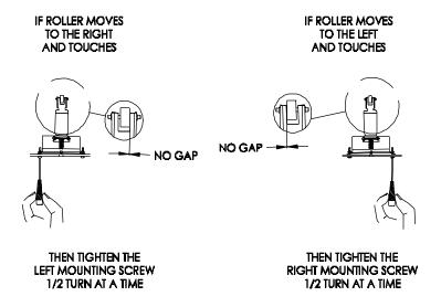
Figure 3-15. Upper Roller Adjustment.
